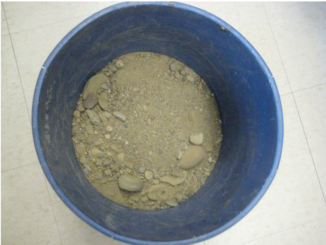
FIGURE 5: The sample collected from the quarry was poorly sorted and unconsolidated.
