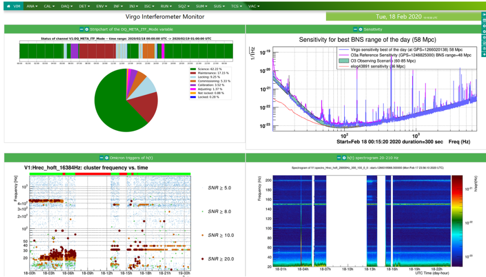
Figure 4. Screenshot of a VIM web page displaying information about the Virgo detector on Tuesday 18 February 2020. Top left plot, stripchart of the detector status: the weekly maintenance, preceded by a planned calibration and followed by a short commissioning period, interrupts the data taking that restarts in the evening. Top right plot: daily sensitivity compared with references. Bottom left plot: glitch monitoring provided by the Omicron analysis described in section 4.1. Bottom right plot: spectrogram of the GW strain h(t) in the 20–210 Hz frequency range.
