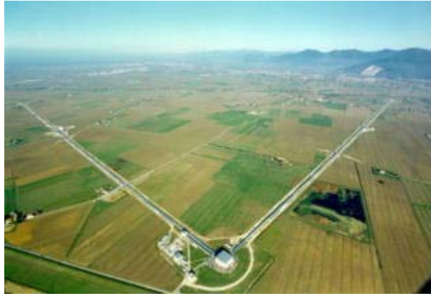
FIGURE 2. External view of the Virgo experiment. The two 3km long arms and the central building are well visible.
