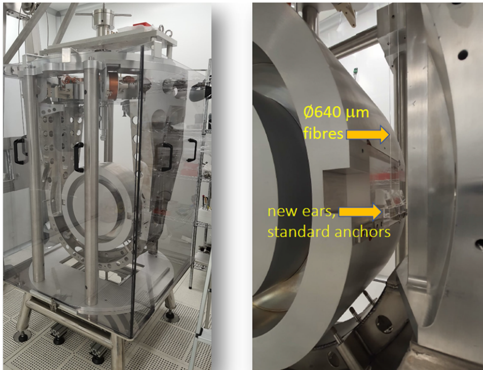
Figure 5. The prototype payload for phase II large masses has been assembled and it is under the test phase, including the 640\ \mu\text{m} thick fused silica fibers which will hold the real mirror.
